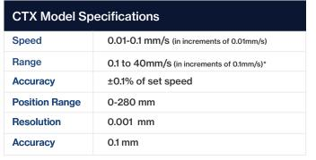
\*Maximum test speed for 100kg = 10mm/s and 50kg = 20mm/s
